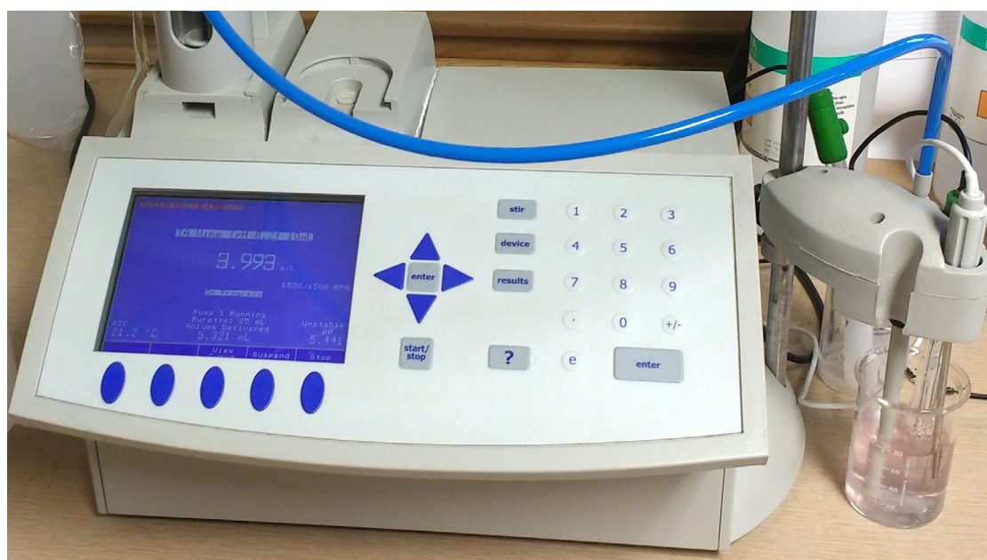
FIGURE 3. A commercially available titrator can measure both pH and acidity levels.
