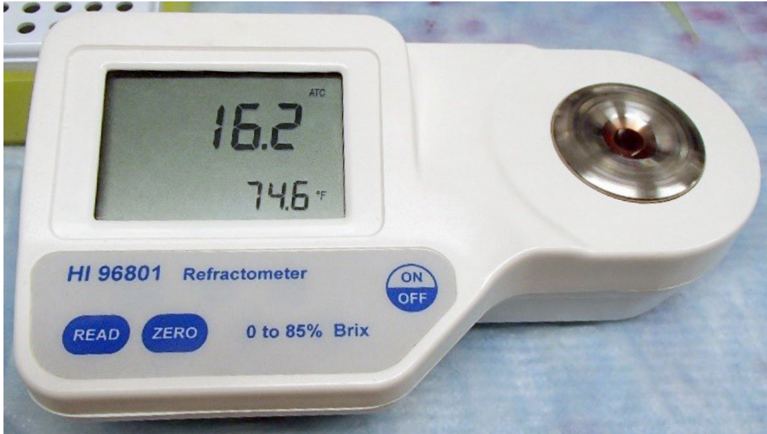
FIGURE 2. A refractometer measures the sugar concentration of fruit juice quickly and easily.
